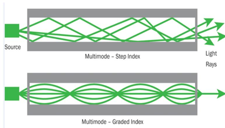
Fig. 2: Types of Optical Fiber
