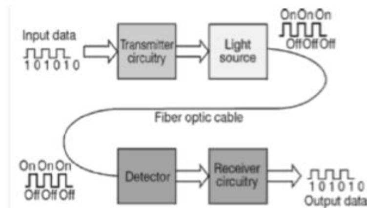
Fig. 1: Block Diagram of Optical Fiber
