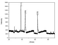
Figure4: X-ray diffraction patterns of synthesized Pt NPs. **4.4 SEM-EDX analysis:**
