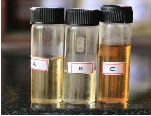
Figure 1. Visual observation of platinum nano particle synthesis (A-Plant extract B-salt solution C- reaction mixture)
