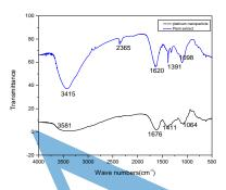
Figure 3: FT IR spectrum of synthesized platinum nano particle of Croton Caudatus Geisel and plant extract
