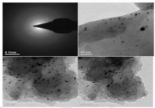
Figure 7: TEM images of platinum nano particles. **4.6 cyclic voltametric analysis:**
