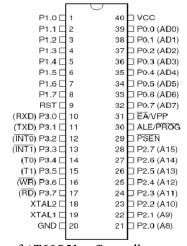
Fig.3.Pin diagram of AT89S51 μ Controller
