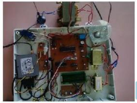
Fig.6. Prototype model of microcontroller based transformer health condition monitoring kit.
