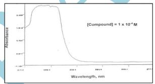
Fig-1: Electronic Spectrum of [Co(enbmo)Cl2]
