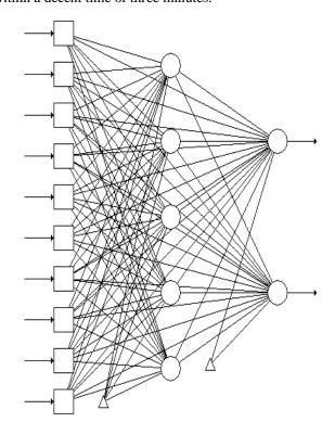
Fig.3 Topology for Feed-forward Neural Network used (10-5-2) in the study
