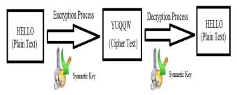
Fig 3: Symmetric key cryptography
