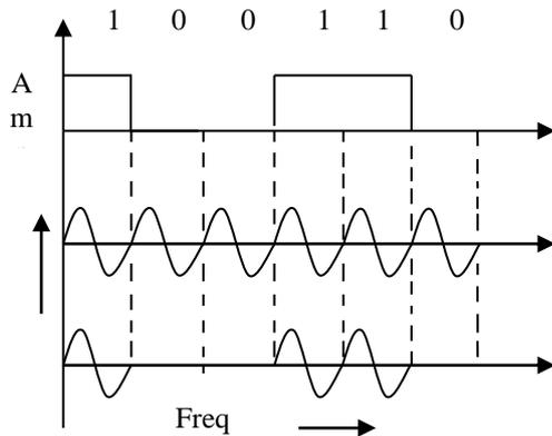
Fig.5: Amplitude Shift Keying
