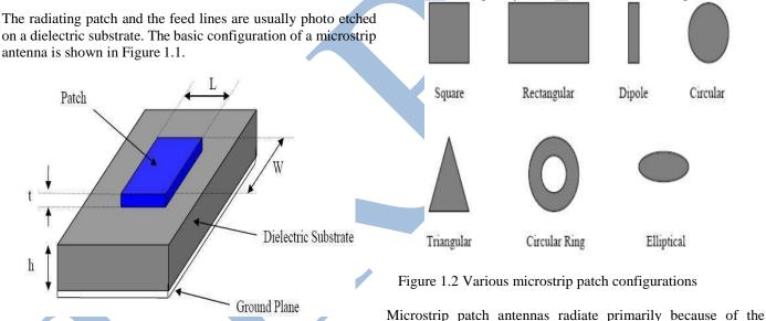
Figure 1.1 Basic configuration of a microstrip patch antenna
