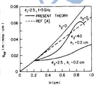
Figure Variations of space wave conductance's with substrate and dielectric thickness (a = 1.1 cm, f = 5 GHz)
