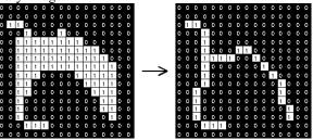
Fig. 1.6: Thinning of a simple binary shape, using the above structuring elements.
