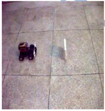
Object from the original frame has been taken and global threshold procedure is used manually to select the best possible threshold value which gives exact number of pixels composing the object
