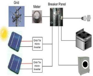
Fig 1.1: Schematic diagram of a simple photovoltaic system
