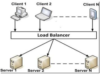
A load balancer is a device that acts as a reverse proxy and distributes network or application traffic across a number of servers. Load balancers are used to increase capacity (concurrent users) and reliability of applications. Cloud load balancers manage online traffic by distributing workload between multiple
