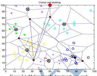
Figure 2.1: Malicious node detection by spy node Figure 2.1 shows the spy node moving on pre assigned path and when it reaches to vulnerable cluster head, a communication link has been setup with that and detection algorithms on spy node decides whether any node is malicious or not. The flow chart for the movement of spy node is shown in figure 2.2.
