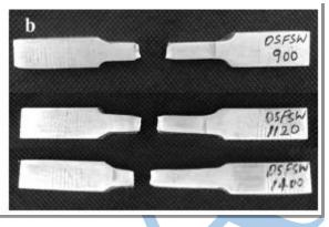
FSW joints at 1120 and 1400 rpm. All the FSW joints failed in the SZ.
