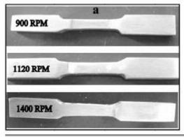
Tensile samples-FSW (a) before testing (b) after testing
