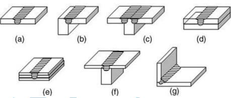
Figure 1.1: Joint configurations for friction stir welding: (a) square butt, (b) edge butt, (c) T butt joint, (d) lap joint, (e) multiple lap joint, (f) T lap joint, and (g) fillet joint.
