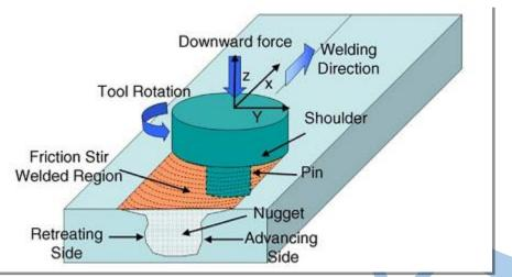
Figure: Schematic diagram of FSW
