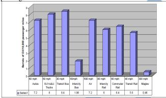
Figure 1: Energy efficiency by transport mode [6]. Source: Transportation Energy Data Book, 25th Ed. By Stacy Davis and Susan Dregel, Center for Transportation Analysis, Oak Ridge National Laboratory, ORNL-6874 (2006) [6].
