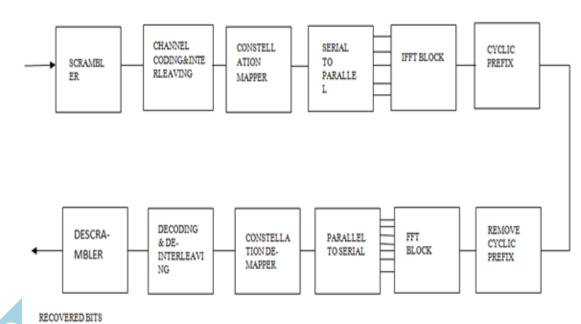
Fig2 Transceiver for 802 11 a
