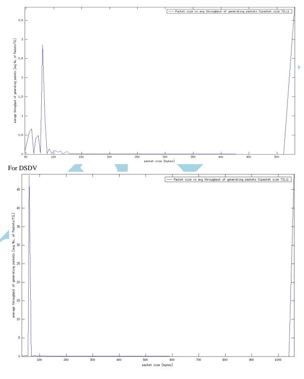
In case of 15 nodes we observe that as the packet size is increasing throughput of dsdv in much higher than olsr.
