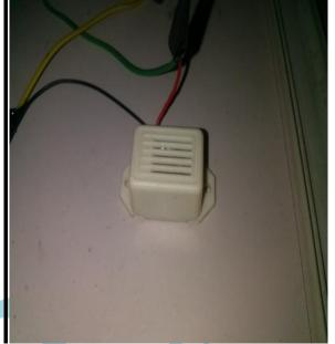
We have used two alarm in this project one is in the engine room and another is in the railway control room. So that train driver and observer in control room are able to show the output and they can take action according to the fault.
