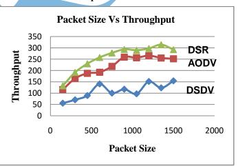
Graph 5.2: Throughput versus Packets sizes for different Protocols
