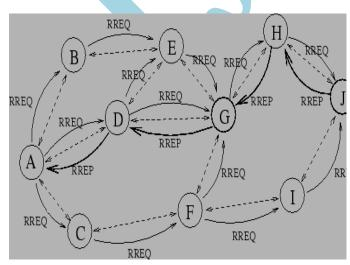
Figure 2: A possible path for a route reply if A wishes to find a route to J.
