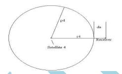
A satellite's position and distance from the receiver define a spherical surface, centred on the satellite. The position of the receiver is somewhere on this surface. Thus with four satellites, the indicated position of the GPS receiver is at or near the intersection of the surfaces of four spheres. (In the ideal case of no errors, the GPS receiver would be at a precise intersection of the four surfaces.)
