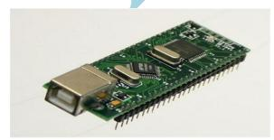
Each pins in the ports can be used as either input or output pins.Before using the port pins as input or output, directions should be given in TRIS register. For example setting all the bits in TRIS D register indicates all the pins in PORT D are used input pins. Clearing all the bits in TRIS D register indicates all the pins in PORT D are used as output pins. Likewise TRIS A, TRIS B, TRIS C, TRIS E registers available for PORT A, PORT B, PORT C and PORT E.
