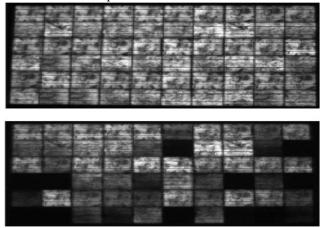
Figure 2: EL image of a panel before (upper) and after (lower)
