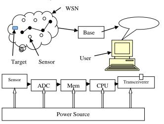
Fig. 1: Wireless Sensor Network
