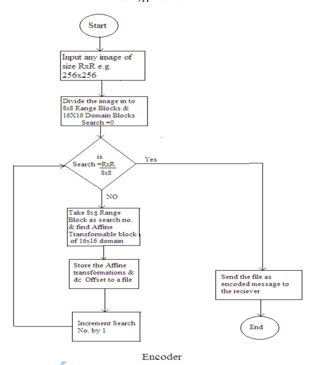
Fig 5: Fractal Image Encoding Block diagram
