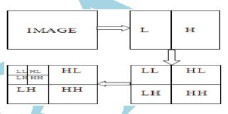
Figure 1. Two levels Wavelet Decomposition applied on an image
