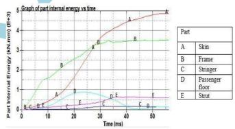
Figure 9: Part internal energy vs time for V= 10 m/s on rigid
