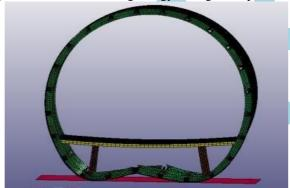
Figure 6 : Deformation for Impact at V=7m/s on rigid
