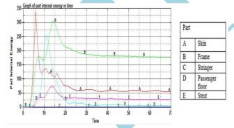
Figure 12 : Part internal energy vs time for V=7m/s on water
