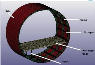
Figure 2 : Fuselage components
