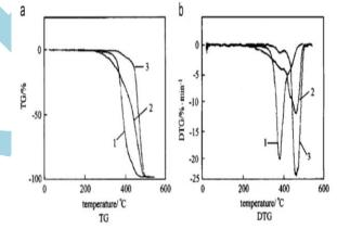
Figure 4.3 The pyrolysis TG and DTG plots of rubber materials.
