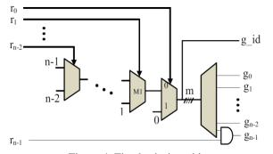
Figure 4. Fixed priority arbiter **B. The mechanism of Variable Priority arbiter**
