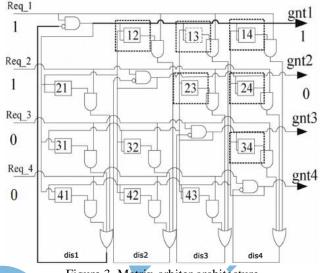
Figure 3. Matrix-arbiter architecture
