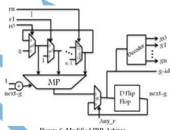
Figure 6. Modified IRR Arbiter IV. ANALYTICAL COMPARISION
