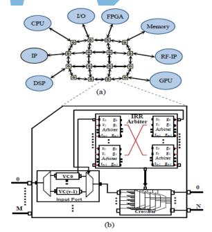
Figure 1. (a) 2D SoC mesh. (b) NoC router.
