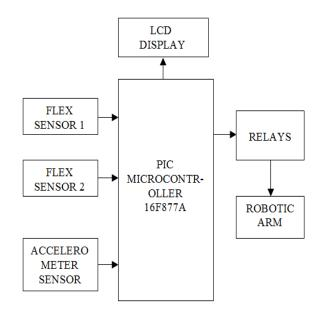
Fig1. Flex sensor based robotic arm using micro controller
