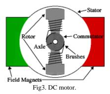
Every DC motor has six basic parts -- axle, rotor (a.k.a., armature), stator, commutator, field magnet(s), and brushes. In most common DC motors (and all that Beamers will see), the external magnetic field is produced by high-strength
