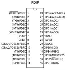
A low power of CMOS 8 bit microcontroller based on the AVR RISC architecture. By executing powerful instruction in a signal clock cycle. at the ATmega8 achieves throughputs approaching allowing the system . Voltage regulators keep a constant dc output despite input voltage or load changes. The two basic categories of voltage regulators are linear and switching. The two types of linear voltage regulators are series and shunt. The three types of switching are step-up, step-down, and inverting.
