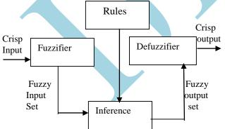
Fig.3. Components of Fuzzy block system.
