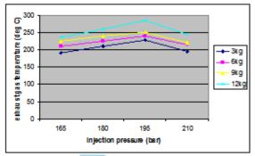
Fig 10. Variation of T<sub>exg</sub> with Injection Pressure (B10)
