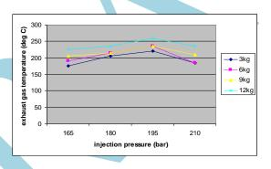
Fig 11. Variation of T<sub>exg</sub> with Injection Pressure (B20)
