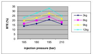
Fig 1. variation of BTE with Injection Pressure (100% diesel)
