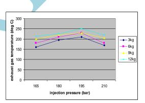
Fig 12. Variation of T<sub>exg</sub> with Injection Pressure (B30)
