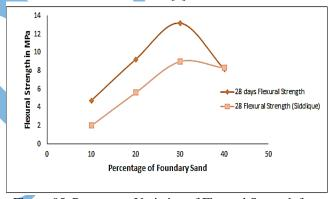
Figure-05. Percentage Variation of Flexural Strength for different foundry sand contents [3]
