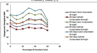
There is increase in compressive strength of cubes and cylinder at 25 to 30% replacement of foundry sand with fine aggregate, after 30% replacement the compressive strength of cubes and cylinder is start decreasing. As the duration increases the compressive strength is increasing. The highest compressive strength is observed at 30% replacement at 28 days and it is up to 50 to 55 Mpa [3].
