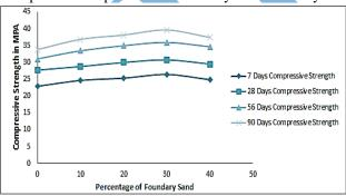
Figure-02. Compressive Strength and Percentage of Foundry Sand [4]
