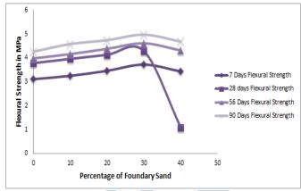
Figure-04.Flexural Strength and Percentage of Foundry Sand [4]
