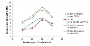
Figure-03. Percentage Variation of Compressive Strength for different foundry sand contents.[4]
